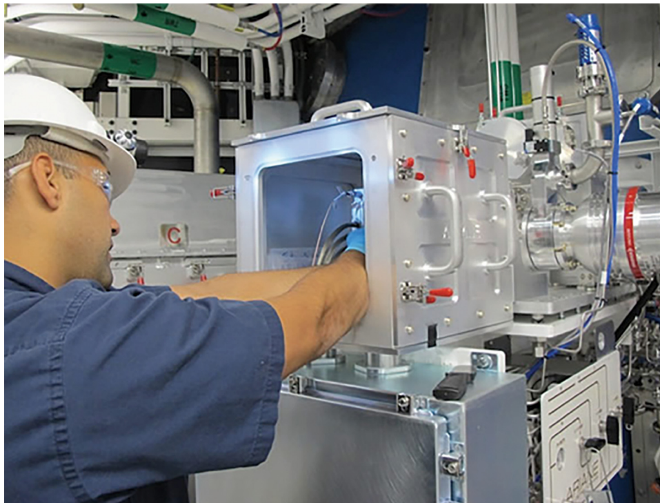
Fig. 11. A technician installs a film pack in the ARIANE GXI for an experiment. ARIANE uses a CCD detector to electronically capture and record X-ray data for higher-yield experiments.
