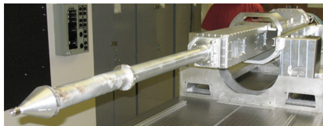
Fig. 7. Hardened gated X-ray imager with imaging snout attached. The hGXI is the rectangular box at the back. The pinhole assembly at the front (left) end of the snout is typically located 8 to 10 cm from the target.
