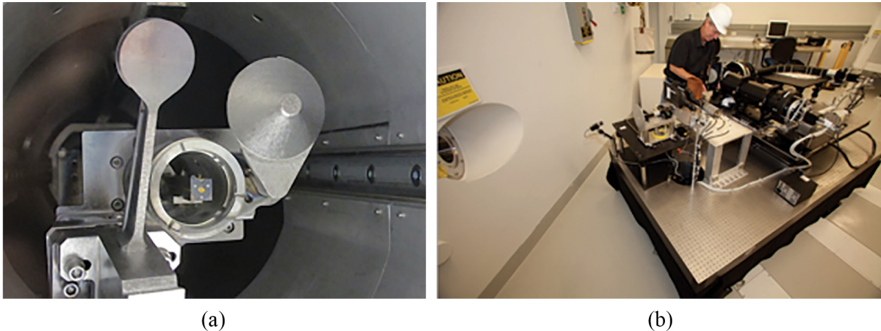
Fig. 12. (a) The front end of the NIS. The square object in the middle is the front end of the neutron pinhole array. The round object on the right is the debris shield in its open position to allow alignment. The other round object on the left is the converter foil for the MRS (Sec. III.C.2). (b) The detector end of the NIS located 28 m from the TCC. The neutrons travel from left-to-right through the detector system.
