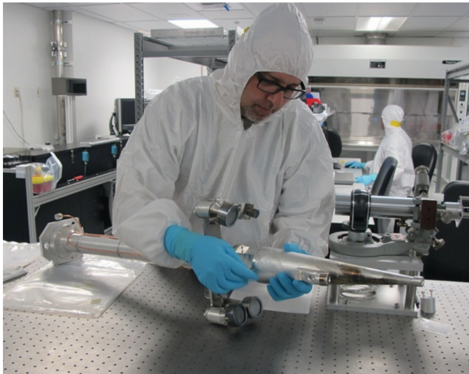
Fig. 8. The PTOF detector is mounted on the side of the X-ray imaging snout. Here, a technician assembles a snout supporting three SRC detectors (top left and bottom) and a PTOF detector (top right) for an experiment. PTOF determines the timing of fusion production using a diamond detector that responds to neutrons and protons. The end of the snout has a pinhole array that is inserted on a DIM to \sim 10 cm from the NIF implosion. The assembly shown in this figure is attached to an air box that has a time-resolved detector such as a GXD or a DISC.
