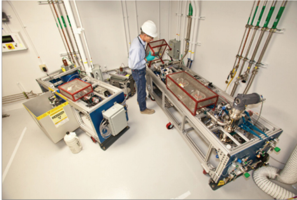
Fig. 14. The RAGS system collects and analyzes gases produced by NIF experiments.
