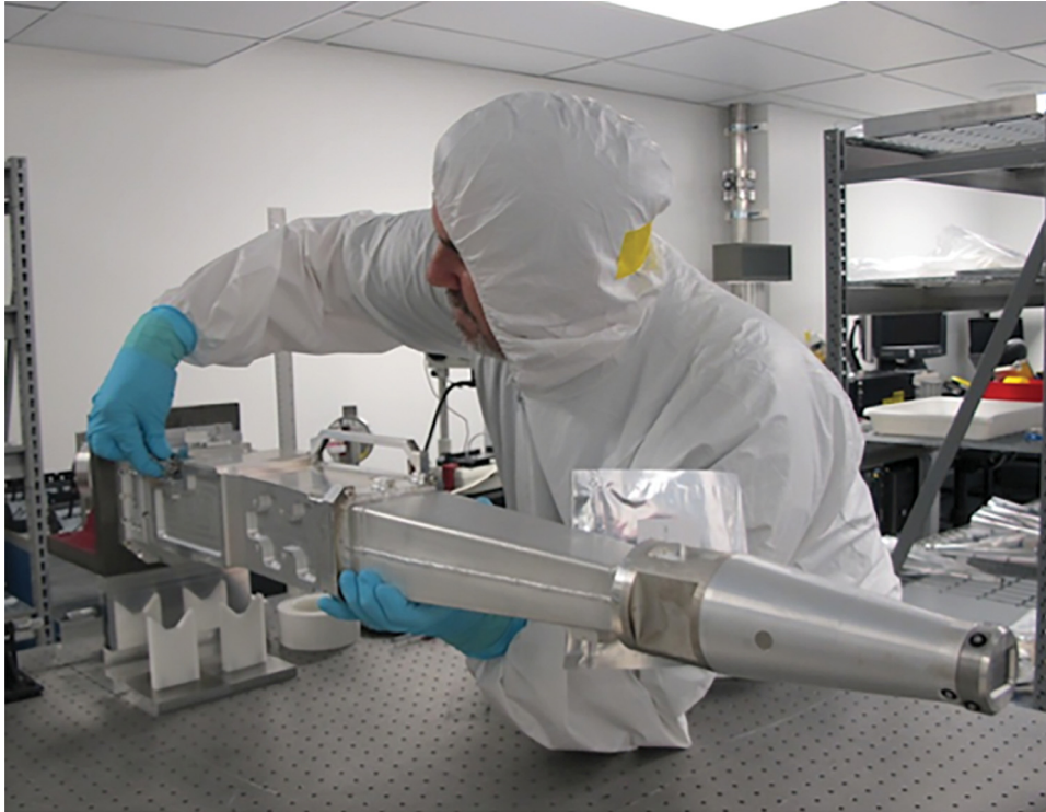
Fig. 16. The Super-snout four-channel crystal spectrometer is attached to the recording box.
