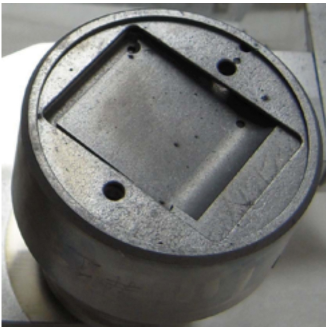
Fig. 15. The WRF detector unit. The rectangle is a wedge of aluminum covering the plastic detector, which is CR-39. The cassette shown has a diameter of \sim 3 cm.
